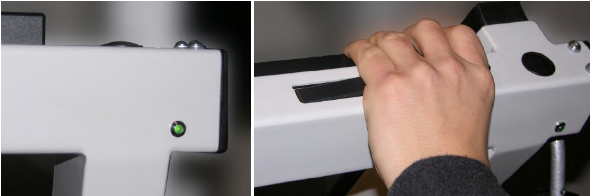
Illustration 6.6: left: Phoropter with green LED; right: Phoropter tilted, LED off
